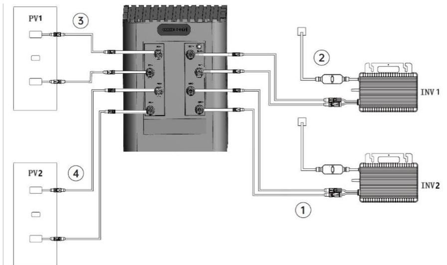
Figure 3-4 System Installation Schematic Diagram
