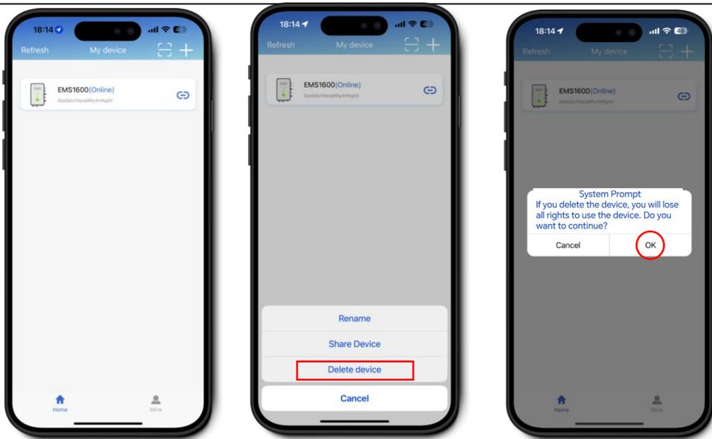
Figure 5-5 Device Deleting
