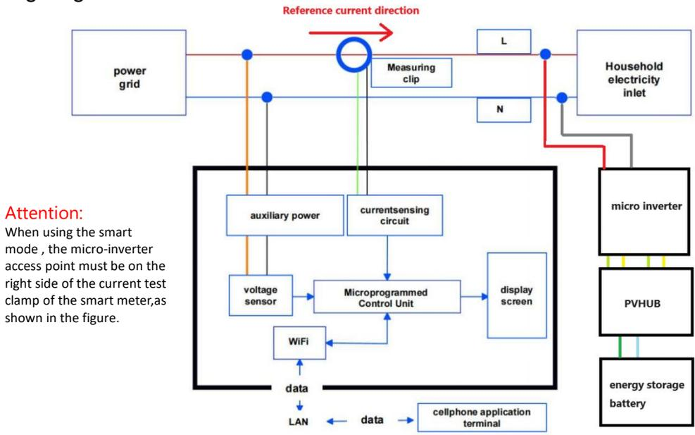
Figure 3-4 Wiring Diagram of the Smart Power Meter
