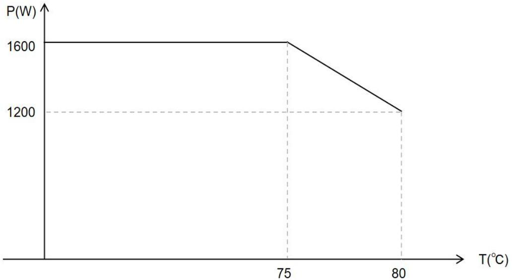
Figure 4-6 Power Derating Curve Graph
