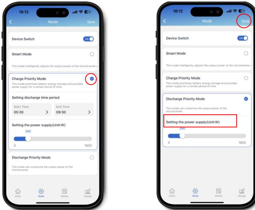
Figure 5-4-3 Discharge Priority Mode Setting
